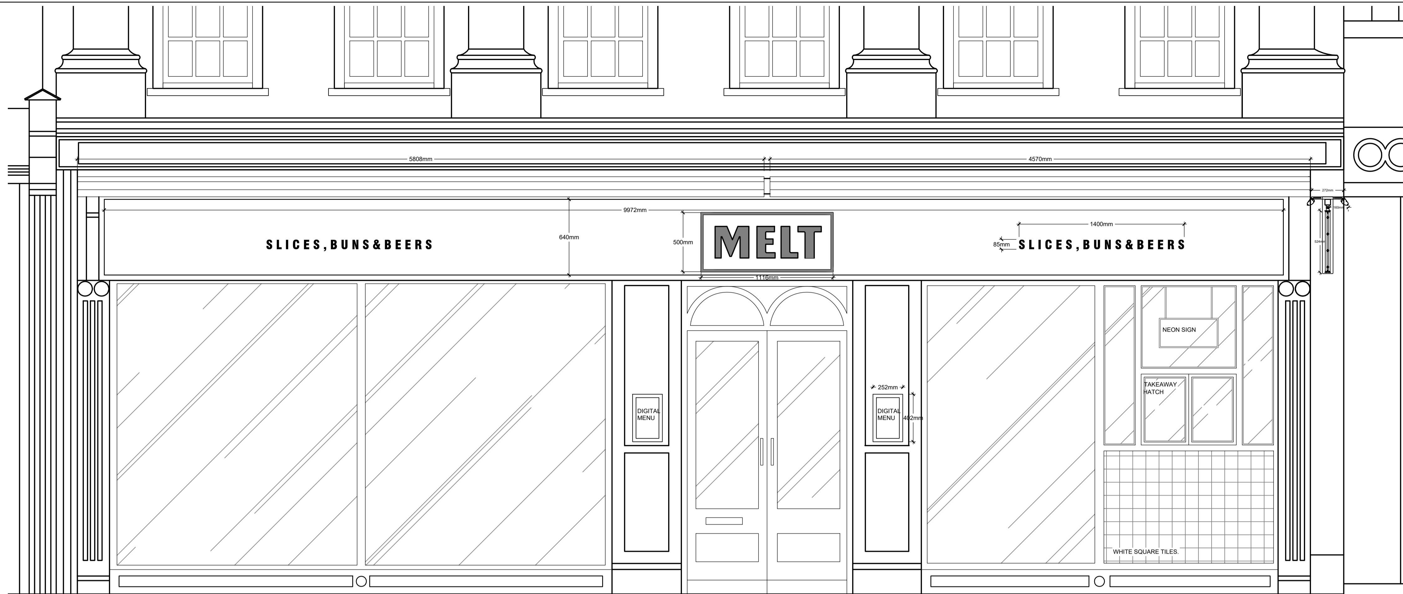
PROPOSED EXTERNAL SIGNAGE ELEVATION SCALE: 1:20
