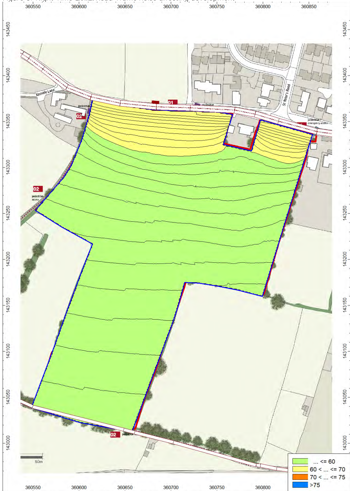
Figure 6: Night Time LAF max Road Traffic noise affecting development
