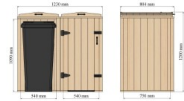
Bellus Double Wheelie Bin Storage for 1 x 180 Litre Bin and 1 x 140 Litre Bin Dimensions
