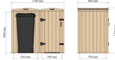
Bellus Double Wheelie Bin Storage for 1 x 240 Litre Bin and 1 x 180 Litre Bin Dimensions
