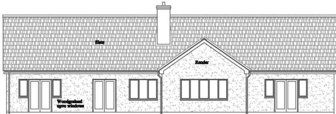
SOUTH WEST ELEVATION
