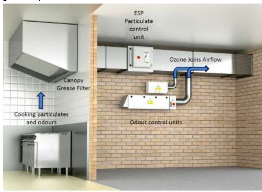
Figure 14: Odour control scheme employing an electrostatic precipitator, operating alongside grease separation and UV-C/Ozone
