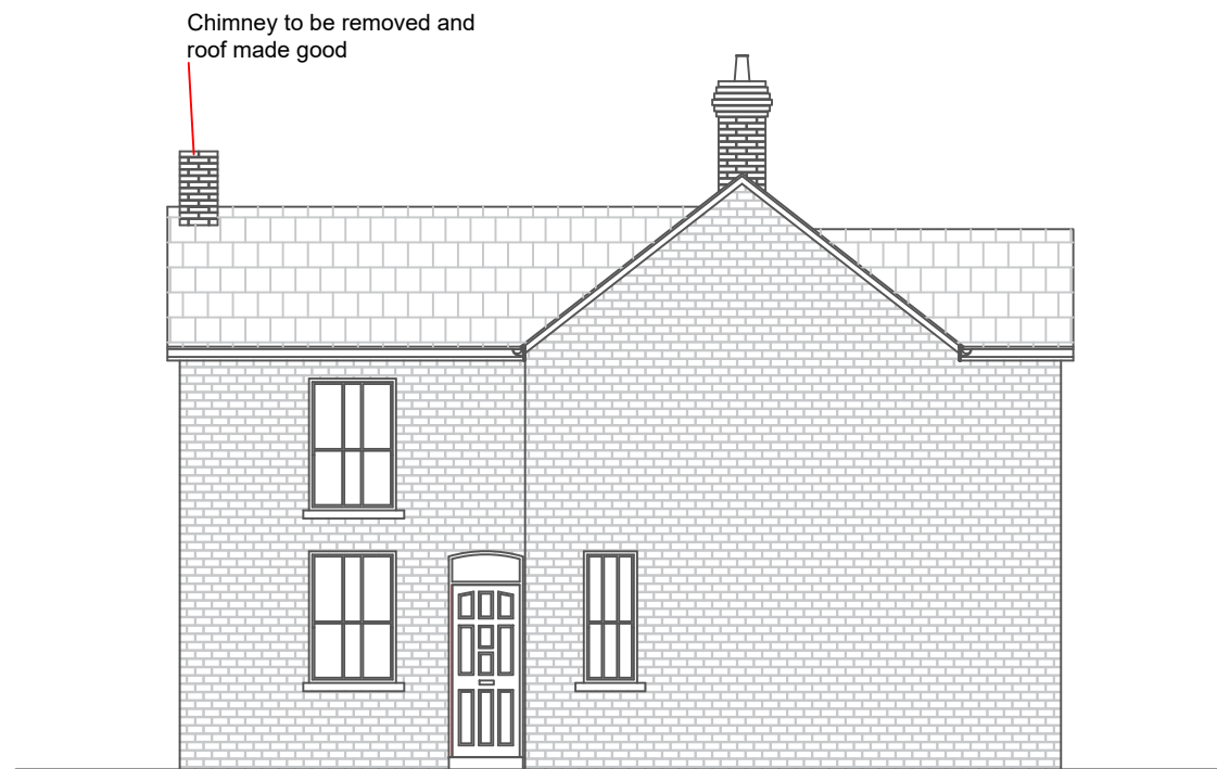
Side (North) Elevation
