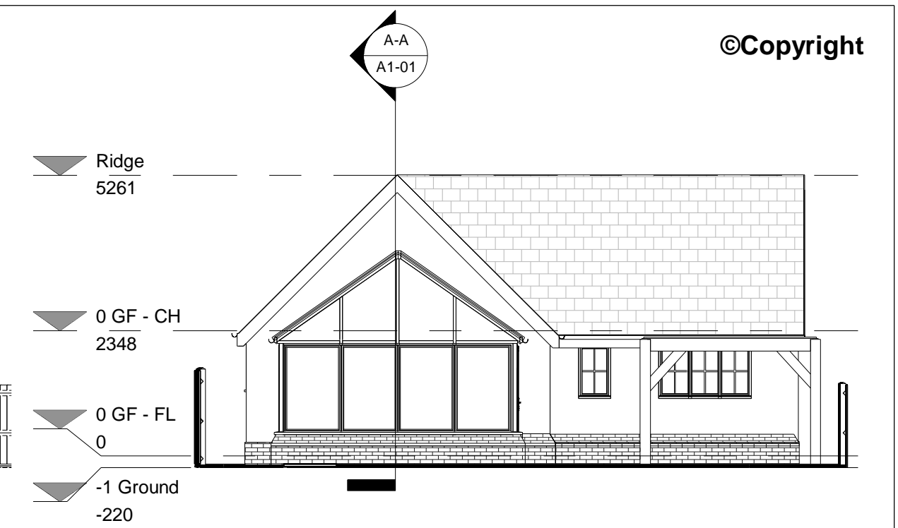
Existing Rear Elevation 1 : 100
